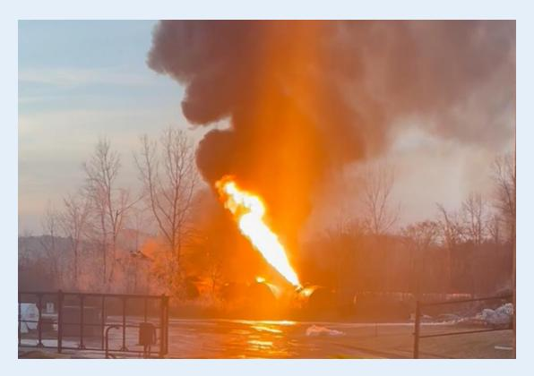
After releasing material, the PRD Closed and Remained Closed (Source: NTSB)
